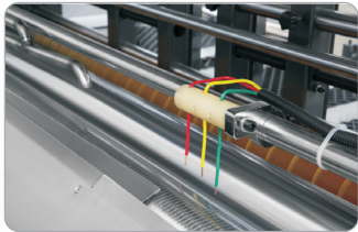
自动胶水补充，网纹辊涂胶 Gluing system
